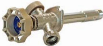
FIGURE: M72AS ▪ 1/2" Sweat x 1/2" IPS Male ▪ Anti-Siphon ▪ ASSE certified 1019 ▪ Built-in Vacuum Breaker
